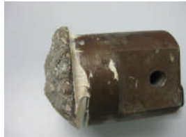
Concrete pulled out of Substrate at 464 psi
